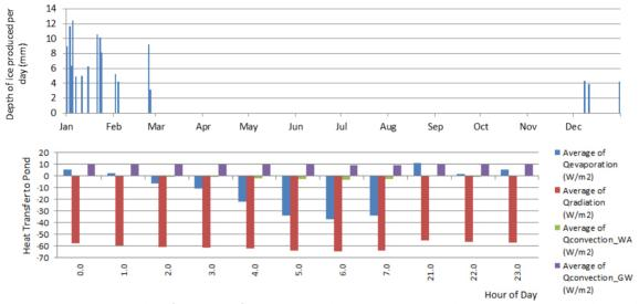
Figure 5. Model results of heat transfers in the Meybod ice pond. The values are the average value at the stated time for all the days of the coldest week.
